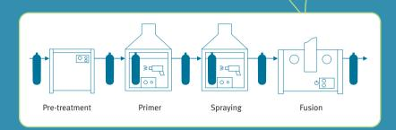
\* Depending on the desired coating thickness and the nature of the metal, the time and / or temperature in the oven may vary. For further information, please refer to the Technical Datasheets on the processing of Rilsan® Fine Powders.
